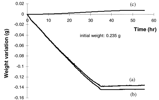
Fig. 9. Oxidation by oxygen at 1470 K: (a) overall weight variation, (b) weight loss due to carbon gasification, (c) weight gain due to SiC oxidation.
